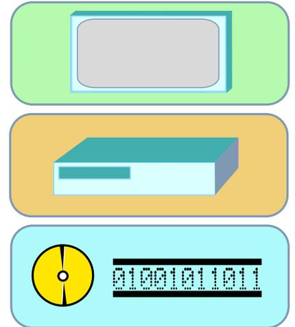
In its simplest implementation, a digital signage installation includes a content stream (from a CD, DVD or the Internet), a playback device, and a display (e.g. a television, plasma display, or LCD panel).
