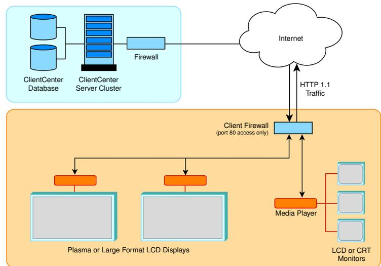
Remote management tools like WireSpring's ClientCenter service allow signage administrators to control media players located in remote networks via the Internet – even when the players are behind firewalls and other perimeter security devices.
